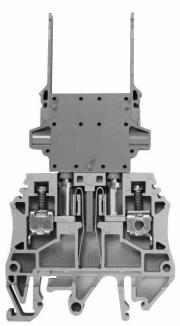
Disconnect test terminals are put to use in all kinds of applications where it becomes necessary to tap into the electrical circuits for test and control purposes. In order to perform the measuring procedure as quickly as possible, the test adapter must be quick and easy to connect. Together with the corresponding test adapters, the new WTL 4/2 STB facilitates disconnecting the circuit by opening the busbar and connecting to the test sockets in a single movement.
